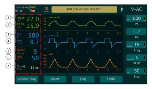
FIGURE 46 Ventilation Parameters
